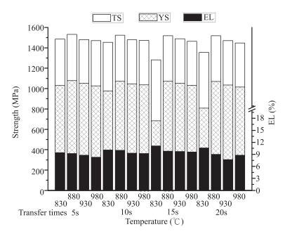
**Fig.13.** Strength and elongation for 15B22 (t = 2 mm) at different temperatures and transfer times under 25 tons pressure.
