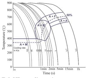
**Fig.8.** CCT curves of hot stamping process temperature vs. time with various cooling rates<sup>(6)</sup>.
