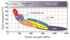
**Fig.1.** The elongation vs strength of different steel materials<sup>(1)</sup>.
