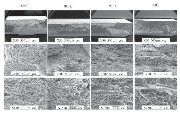
Fig.14. SEM analyses of cross-sectional tensile specimens of 15B22 after die quench.
