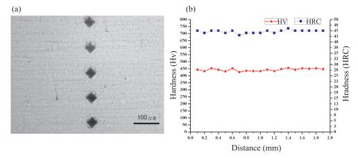
**Fig.11.** The hardness of 15B22: (a) indentations on the specimens; and (b) variation of the micro-hardness (Hv) and the Rockwell hardness (HRC). Test conditions of hardness: loads of 500 g (Hv); 15B22 heating to 830°C; and a 5 second transferral to die quench under 15 tons pressure.
