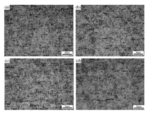
**Fig.15.** The microstructure of 15B22 after heating to 880°C followed by sending the specimen to the mold under 25 tons pressure die quench in time: (a) 5s; (b) 10s; (c) 15s and (d) 20s
