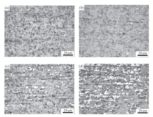
**Fig.9.** The microstructure of 15B22 after heating to 830°C and sending to the mold under 15 tons pressure at different times (a) 5s; (b) 10s; (c) 15s and (d) 20s.
