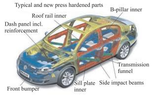
**Fig.3.** Hot stamping parts for automotive applications in a  $car^{(2,3)}$ .
