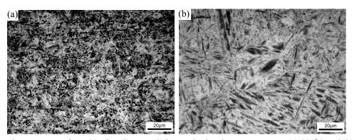
Fig.17. The microstructure of 15B22 after die quench from prior heating temperatures (a) 880°C and (b) 930°C.
