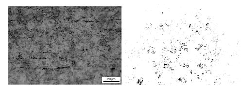
Fig.16. The microstructure of 15B22 heating to 880°C and sending to the mold in 20 seconds after die quench.
