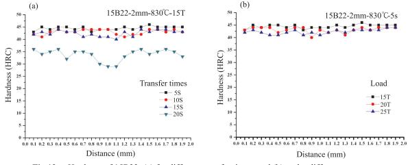
Fig.12. Hardness of 15B22: (a) for different transfer times; and (b) under different pressures.
