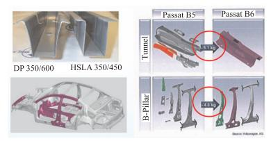
Fig.2. High strength steels in vehicles with improved safety and light weight<sup>(1)</sup>.
