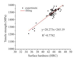
**Fig.18.** Relationship of hardness and strength for hot stamping steel after die quench.
