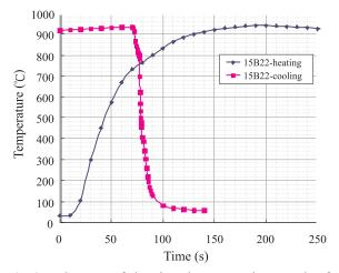
**Fig.6.** Curves of heating hot stamping steel of 15B22 (t = 2mm) to  $930^{\circ}C$  and that of cooling after die quench.
