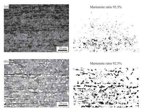
**Fig.10.** The microstructure of 15B22 after heating to 830°C followed by sending the specimens to the mold under 25 tons pressure die quench in transfer times (a) 5s; (b) 10s.
