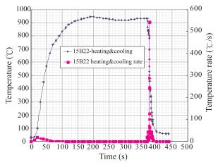
**Fig.7.** Curves of heating and cooling temperature as well as instantaneous rate of 15B22 as heating to  $930^{\circ}$ C followed by cooling after transferral to die quench.
